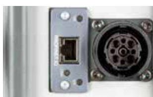
RCI 4 ANYBUS robot interface (built in Sigma Select)
